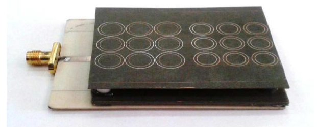
Fig 3: Prototype of the fabricated antenna in Fig 1(b), they have the required distance [7]
