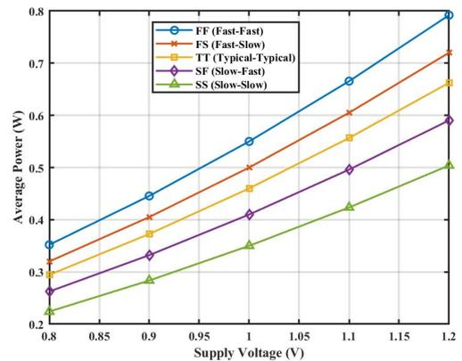
Fig. 21. PVT analysis of average power versus supply voltage (0.8 V to 1.2 V).
