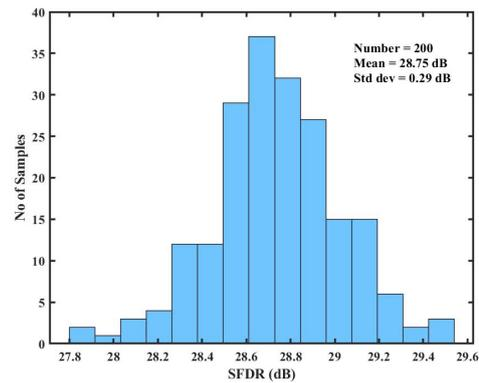
Fig. 15. Monte-Carlo analysis of SFDR with an input signal frequency of 1.36 MHz at 200 MS/s.
