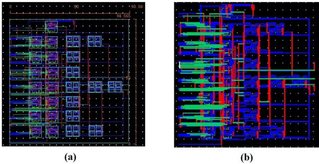
Fig. 19. Layout of 4-bit flash ADC (a) Pre-layout (b) Post-layout.
