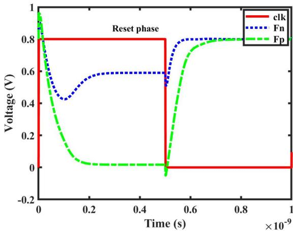
Fig. 4. Transient analysis of pre-amplifier stage DTDC.
