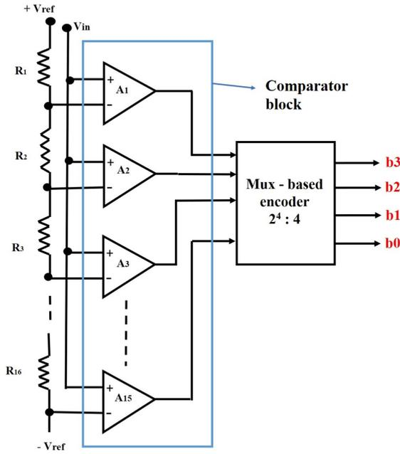
Fig. 1. Architecture of 4-bit flash ADC.
