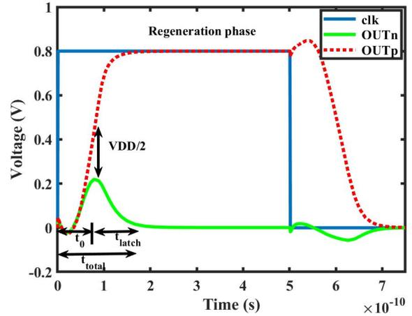
Fig. 5. Transient analysis of Latch stage DTDC.
