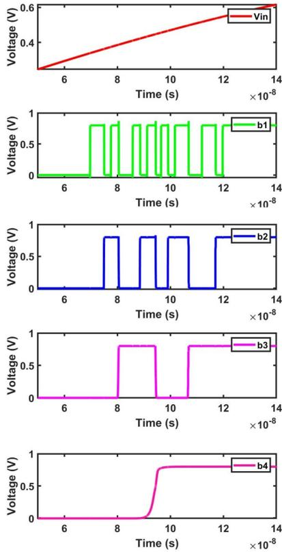
Fig. 7. Transient analysis of 4-bit flash ADC with an expanded output.
