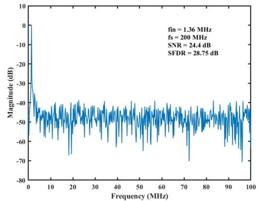
Fig. 10. The output spectrum at a sampling rate of 200 MS/s for input signal frequency of 1.36 MHz.
