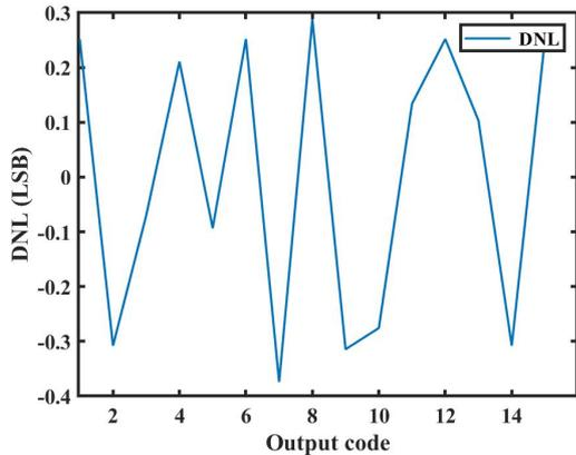
Fig. 8. DNL of 4-bit flash ADC.
