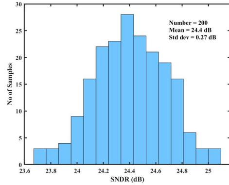
Fig. 14. Monte-Carlo analysis of SNDR with an input signal frequency of 1.36 MHz at 200 MS/s.
