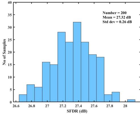
Fig. 17. Monte-Carlo analysis of SFDR with an input signal frequency of 99.41 MHz at 200 MS/s.
