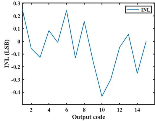
Fig. 9. INL of 4-bit flash ADC.
