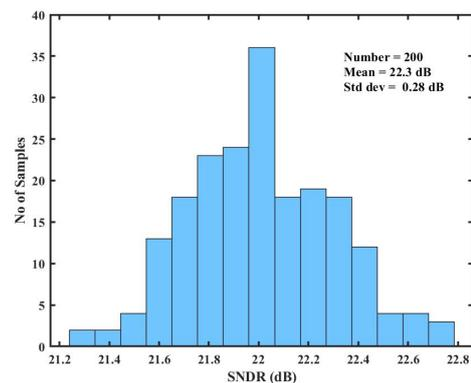
Fig. 16. Monte-Carlo analysis of SNDR with an input signal frequency of 99.41 MHz at 200 MS/s.
