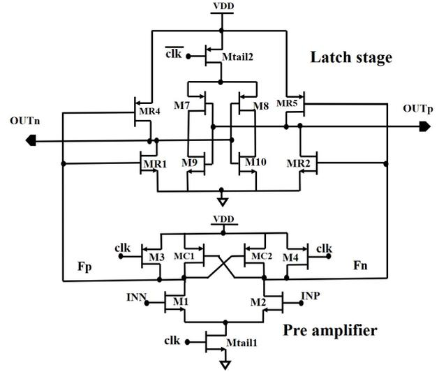
Fig. 2. Low-power double tail dynamic comparator.
