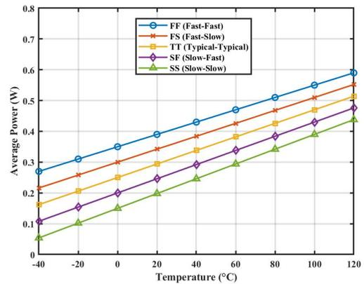
Fig. 20. PVT analysis of average power versus temperatures ( $T = -40^{\circ}$  C to  $120^{\circ}$  C).
