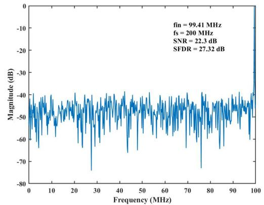
Fig. 11. The output spectrum at a sampling rate of 200 MS/s for Nyquist signal frequency of 99.41 MHz.
