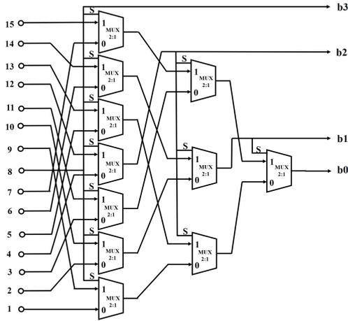
Fig. 3. Architecture of 16:4 bit MUX-based encoder.
