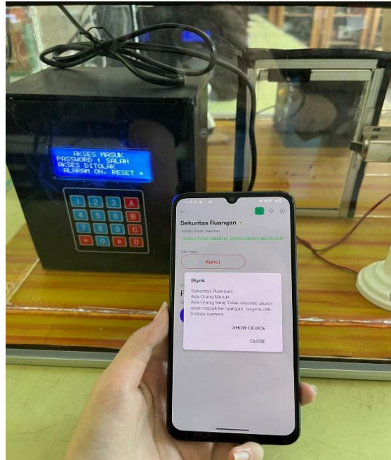
Fig 10: Demonstrates the system’s response when detecting an incorrect password input
