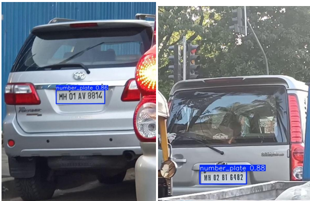
Fig. 2: License plates detected and recognized using YOLOv11 and Easy-OCR.
