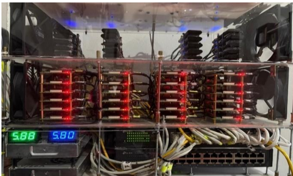
Figure 2: 24-node Raspberry Pi 4B (8 GB) Beowulf cluster architecture for distributed SqueezeNet training.
