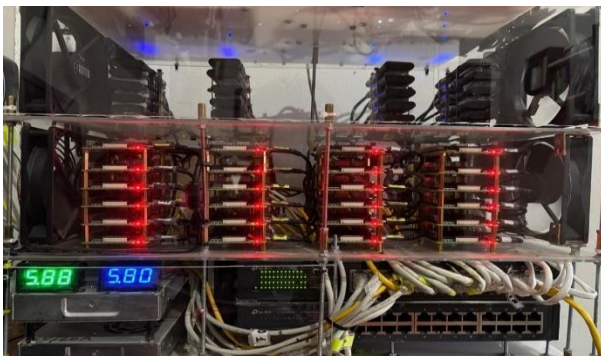
Figure 2: Deployment of the Beowulf Cluster with (24) RPi-4B (8GB).
