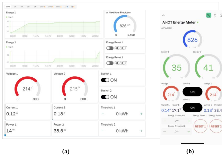
Figure 12: Testing of the developed smart energy meter, screenshot of (a) Blynk webpage, (b) Blynk application interface.
