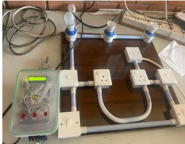
Figure 8: Mobile Phone Enabled Smart Home Automation System with Demonstration Board
