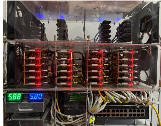
Figure 2: Deployment of the Beowulf Cluster with (24) RPi-4B (8GB).
