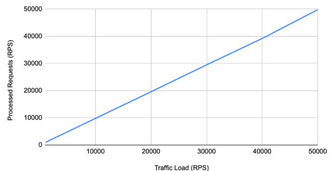
Fig 6. Throughput vs. Traffic Load - Displays the system's capability to handle increasing requests. The results show that the proxy sustains 50,000 RPS, ensuring scalability while enforcing mTLS, JWT authentication, and RBAC.
