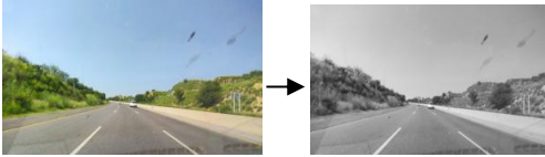
Figure. 6. RGB to grayscale conversion
