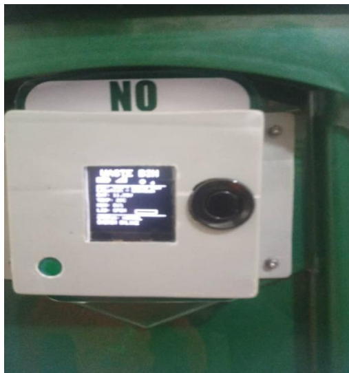
Figure 6: Bin status showing on the OLED display
