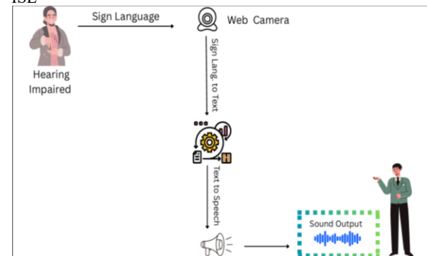
Fig 1: Block Diagram of the Proposed Bidirectional ISL Translation System
