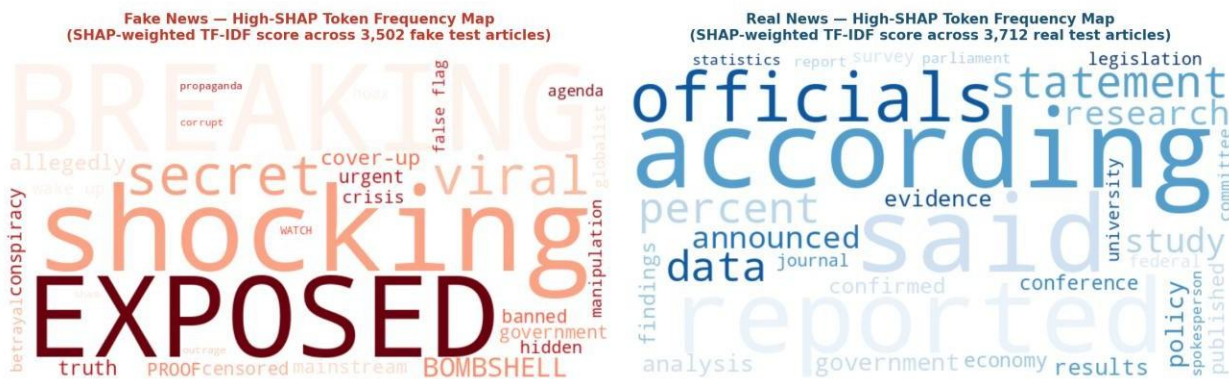
Figure 23: SHAP-Weighted Word Clouds — WELFake Test Set (n=7,214). (Left) Fake-class tokens: token size \propto mean SHAP contribution toward Fake class \times frequency across all Fake test articles; red colour scale with darker = higher SHAP weight. Dominant tokens: BREAKING, SHOCKING, EXPOSED, viral, conspiracy, mainstream. (Right) Real-class tokens: blue colour scale; tokens most predictive of authentic journalism: "according", "percent", "statement", "announced", "research", "study". Stopwords removed; minimum frequency threshold=5. Visualisation generated with WordCloud 1.9 using SHAP-derived weights.
