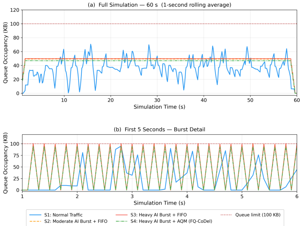
Figure 3 — Queue depth at the bottleneck over the 60 s simulation. Inset shows the burst-idle cycle in the first 5 s.
