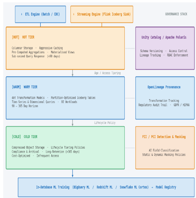
Fig 4: Multi-Tier Storage Architecture and Data Governance Flow within the Intelligent Storage and Warehouse (Layer 3)
