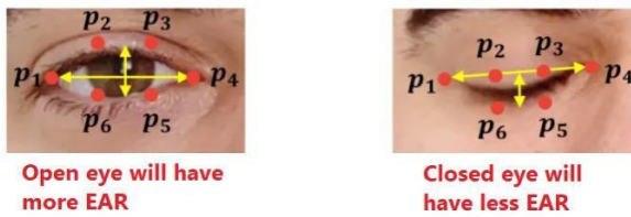
Figure 3: Eye Aspect Ratio (EAR) landmarks showing the difference between open-eye and closed-eye states.
