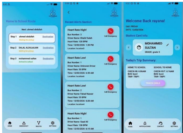
Figure 6: Comprehensive overview of the MUTMA'INN mobile application interfaces. From left to right: (1) Route Tracking Interface, displaying real-time bus stops and student boarding status; (2) Emergency Alerts Section, highlighting critical driver health notifications (Heart Rate Monitoring) with quick-access emergency call features; (3) Main User Dashboard, providing a summarized daily trip log and student identification details.
