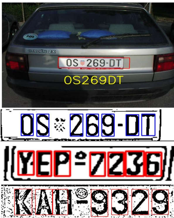
Fig 5: Character Segmentation and Recognition Results showing (a) end-to-end plate detection and recognition, (b)(c)(d) character segmentation and recognition outputs
