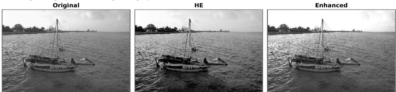
Fig. 1. Visual comparison of the original image, histogram equalization (HE), and the proposed enhanced result
