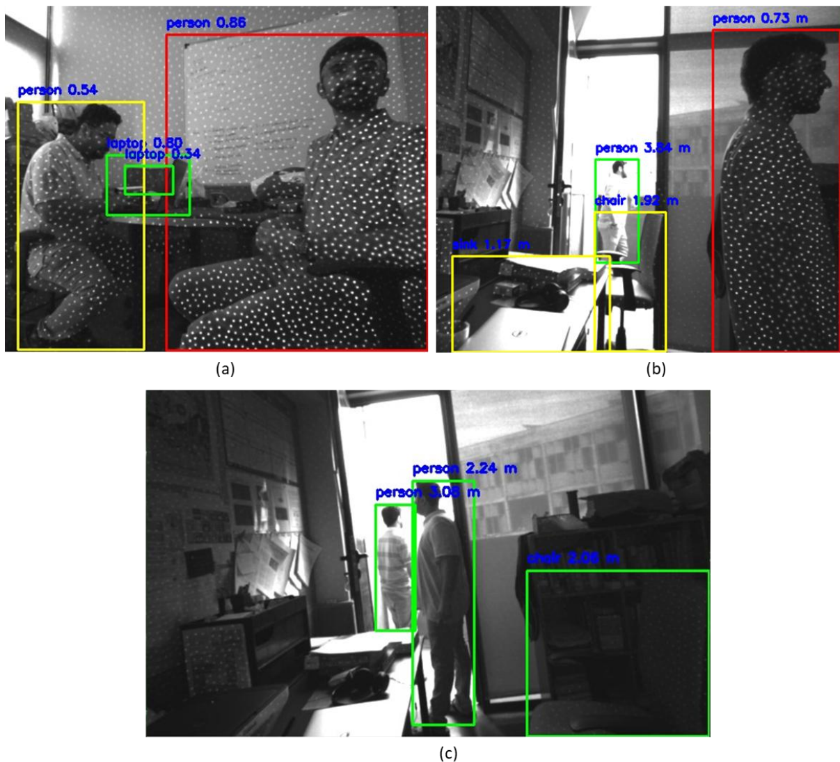
Fig. 10: Camera view from DW2: (a) object identification with confidence value, (b) depth estimation in meters, and (c) a case where all the objects were at a depth of more than 2 m.
