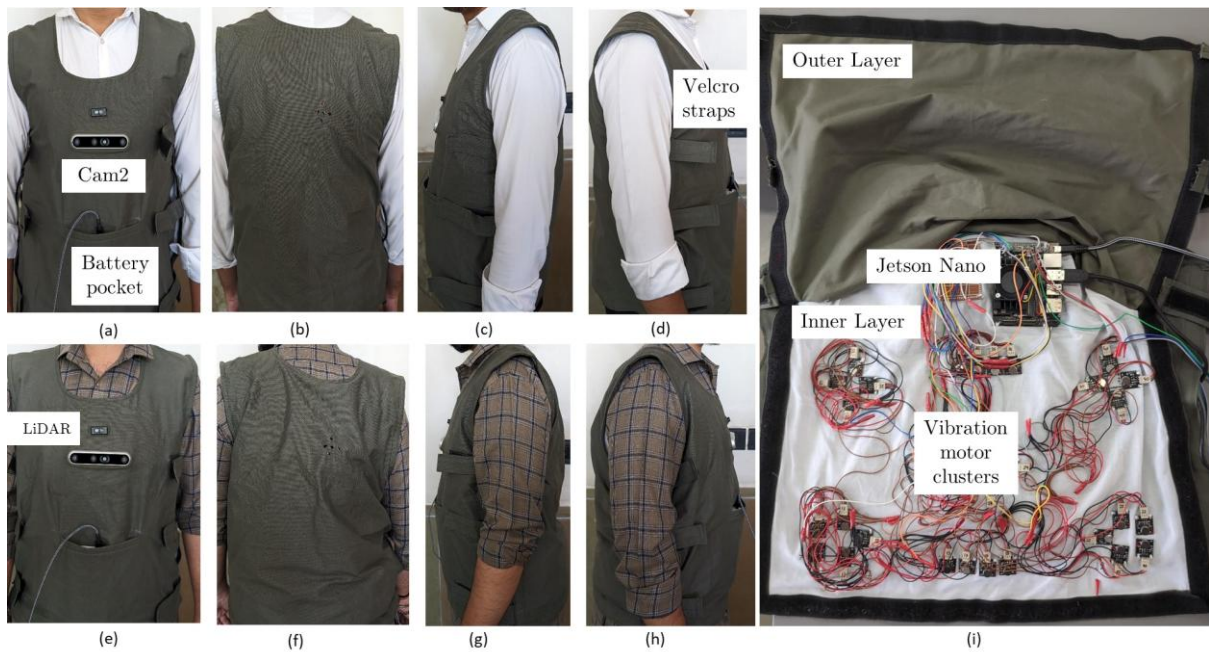
Fig 3: DW-2 prototype; front-back-left-right side views of user 1 (a-d) and user 2 (e-h) wearing DW-2, internal layer of the vest showing vibration motors, connecting wires, and Jetson Nano (i)
