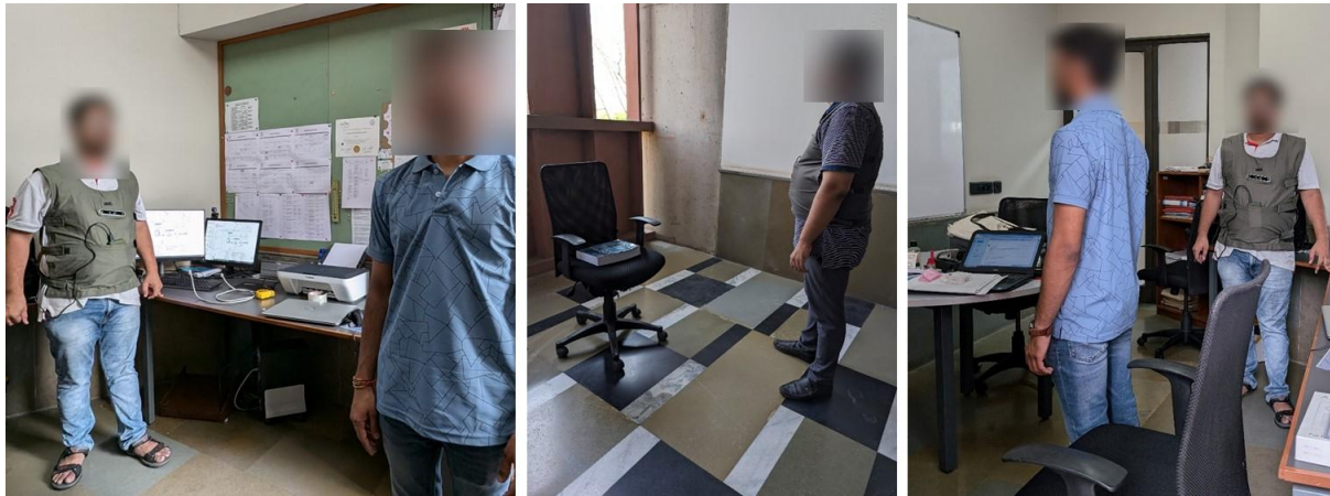
Fig. 9: Testing of DW2: A human in front of the wearer (left), a chair containing book in front of the wearer (middle), and human and chair in front of the wearer (right)
