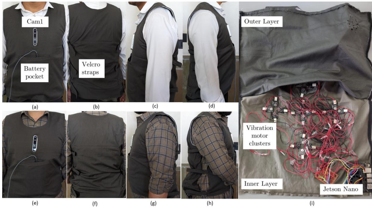
Fig 2: DW-1 prototype; front-back-left-right side views of user 1 (a-d) and user 2 (e-h) wearing DW-1, internal layer of the vest showing vibration motors, connecting wires, and Jetson Nano (i)
