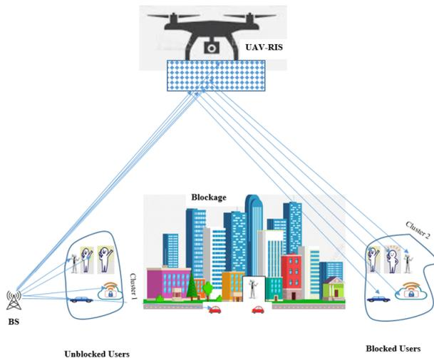
Fig. 1. System Model for RIS UAV mounted RIS
