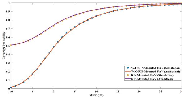
Fig. 7. Comparison of Coverage Probabilities for RIS Mounted UAV and no RIS Scenarios
