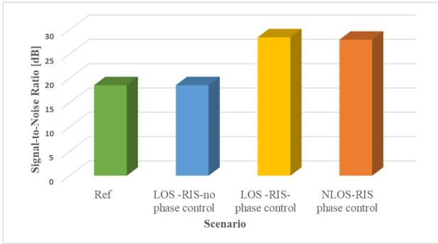
Fig. 6. Effect of RIS Phase Control on SNR
