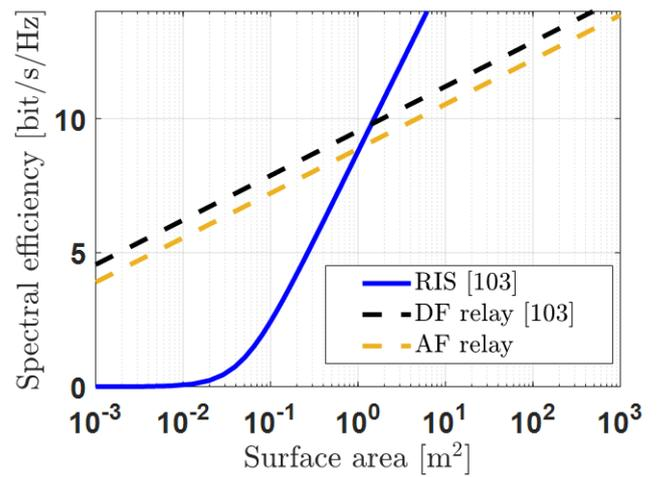
Fig. 5. Effect of Increasing Surface Area of RIS/DF/AF Relay on Spectral Efficiency
