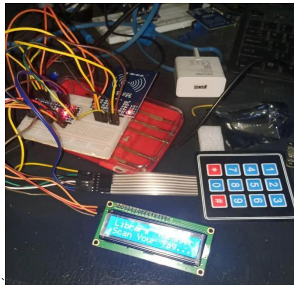
Fig 5: RFID Tag reader Assembled System on Vero board with Circuit cables, Keypad and Tag Reader sensor
