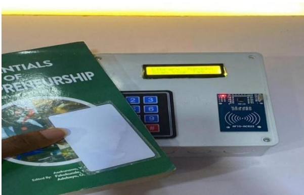
Fig 13: Student using LybSmart RFID Tag Reader to Scan a book tag in the library
