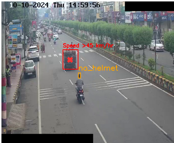
Fig 3: Red Bounding Box for violation due to Over-speeding Frame 2 (Red Cross - Centroid)
