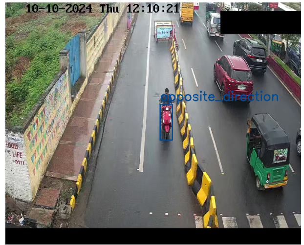
Fig 7. Blue Bounding Box to flag vehicles moving in wrong direction
