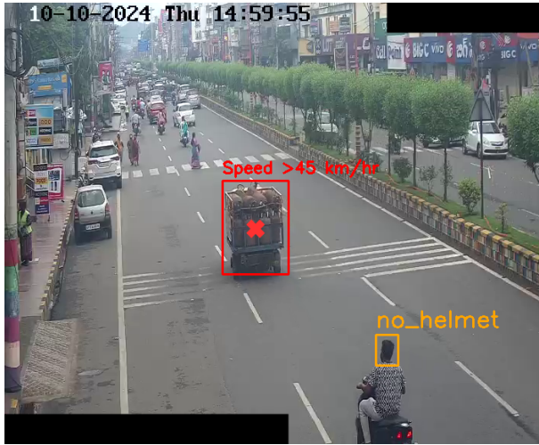
Fig 2: Red Bounding Box for violation due to Over-speeding Frame 1 (Red Cross - Centroid)
