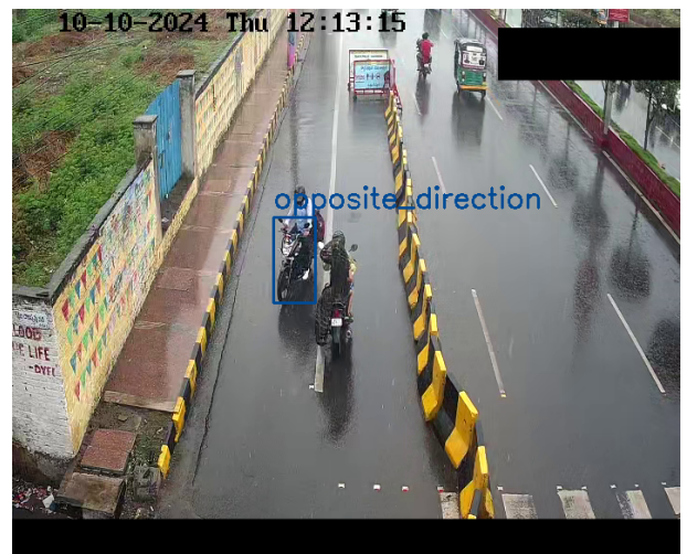
Fig 8. Blue Bounding Box to flag vehicles moving in wrong direction
