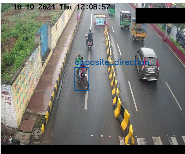
Fig 6. Blue Bounding Box to flag vehicles moving in wrong direction
