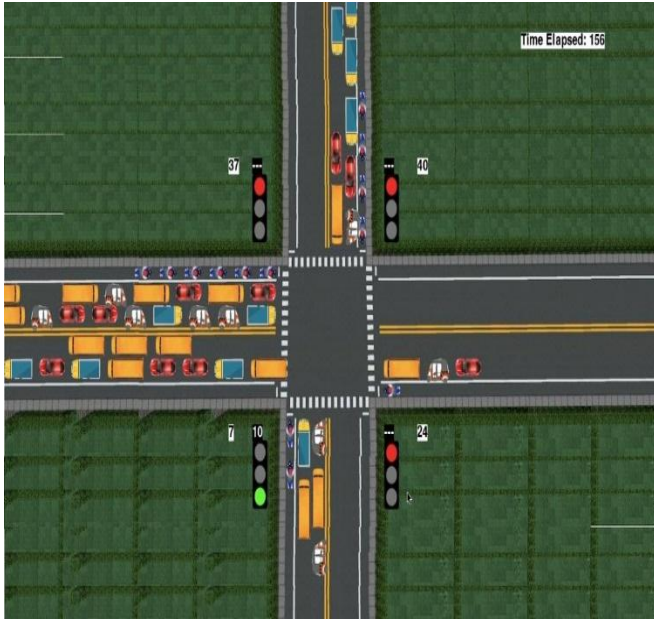
Figure 10: Dynamic adjustment of green signal duration based on traffic volume
