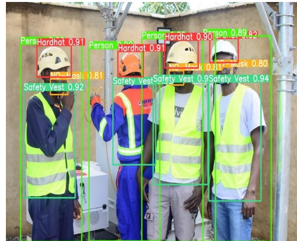
Fig 3: Example showcasing the model's accuracy in identifying PPE items and flagging non-compliance
