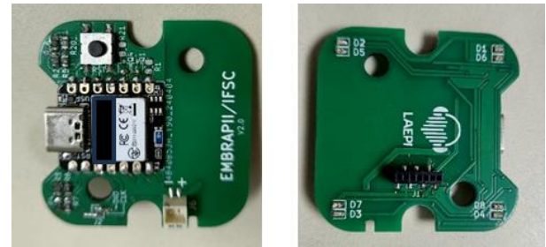
Figure 4. Left: top view. Right: bottom view (microphone PCB connection side) of the mounted main PCB.
