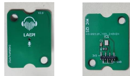
Figure 5. Left: top view. Right: bottom view of the PCB for the PDM microphone.
