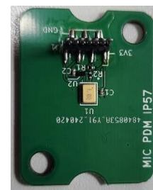
Figure 6. Top view of the PCB for the PDM microphone.
