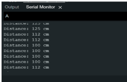
Fig 5: Measured distance after applying the Kalman filter
