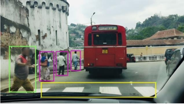
Fig 10: Labelling of the classes (Passenger and zebra crossing) using bounding boxes.
