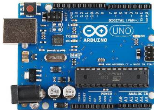
Fig 1. The Arduino UNO board which uses microcontroller ATmega328 onboard.
