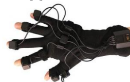
Fig. 2 Setup of sensor-based hand gesture recognition
