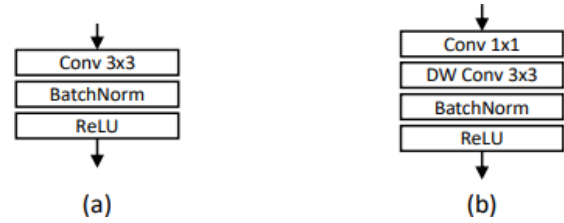
Figure 7: (a) Standard 3 \times 3 convolution (b) Lite 3 \times 3 convolution
